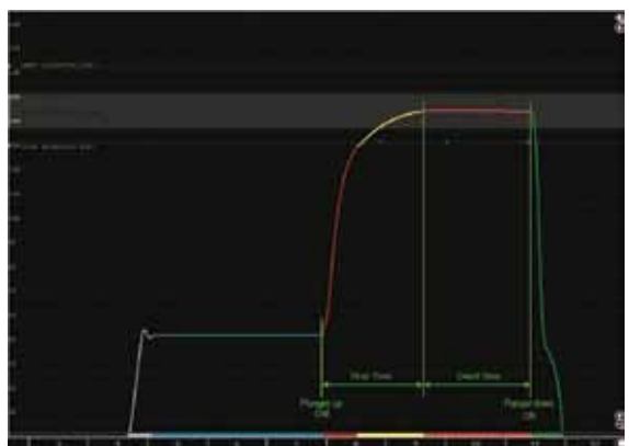
Figure 2: Plunger rise and dwell time between plunger-up and down movement.
