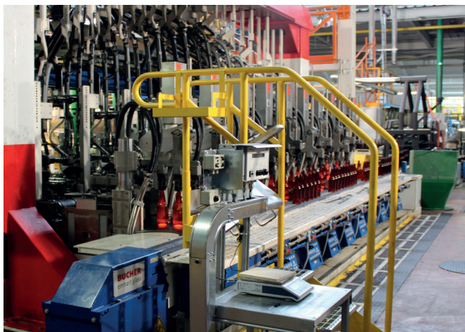
▲ Fig 1. Bucher Emhart Glass's conveyor ladder.
